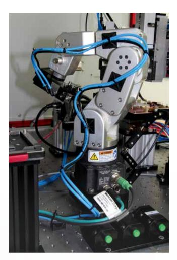
The NanoRobot precisely handles small parts in the VersaWeld station. Repetitive movements are executed with an error of less than 5  $\mu m$ . This performance qualifies the robot for direct placement of workpieces under the weld beam as well as for part inspection in machine vision stations for a visual assessment. NanoRobot has 5 N load capacity and a working range of 300 mm.
