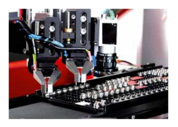
Automated loading of device trays with feeders: Large volume production of TO diode lasers and lens assemblies with stainless steel housings delivered on trays. The dual gripper design reduces the handling time by a factor of 2.
