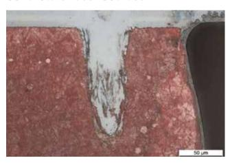
The cross section shows the welding penetration of a Kovar lid to a copper baser with a pulsed fiber laser when purging with protective gas.
