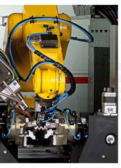
Customized configurations of the VersaWeld System replace tedious manual or semi-automated processes. Robots load the piece parts and can hold them in place during laser welding. With automated seam tracking, the position of the weld beam follows the calculated path for optimum welding results.
