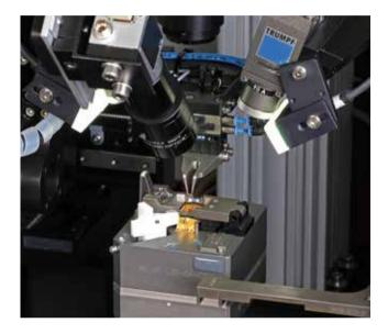
Cameras mounted to the focusing lenses of the laser processing optics support the image data processing during laser soldering and laser welding. Furthermore, machine vision monitors the dispensing of resin or solder paste.
