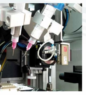
Various assembly techniques can be combined in one station, such as laser welding, laser soldering and epoxy gluing. Exchangeable device trays improve the versatile micro assembly in various batch processes.
