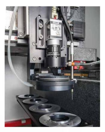
Different toolings can be changed during the process without operator intervention.
