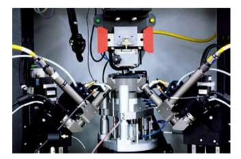
NanoWeld Coaxial A half sphere floating on an air cushion ensures a uniform contact between the two welding surfaces. This results in perfect weld joints with high strength and minimum shift.
