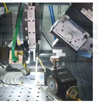
For Silicon Photonics wafers, up to two alignment stacks with 6 degrees of freedom align the optical probes with submicron repeatability. The mounting platform holds the electrical probes which stay in a fixed position after initial manual adjustment.
